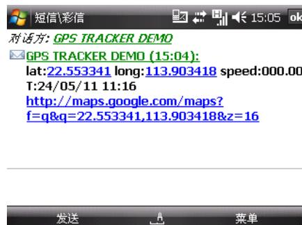
Tracking location , When no GPS signal, the SMS includes the last valid latitude & longitude as well as the LAC code of current position, the LAC code can be input in the column of “manual track” menu of web platform to check location.
